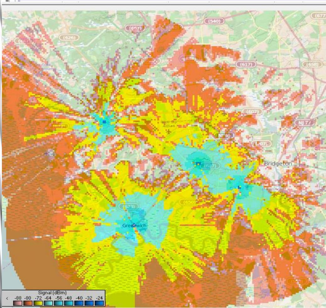
A forecast of potential coverage from four sites, each 50 feet tall, in a gently rolling area of mixed farms, forest, and wetland. Coverage with 70% probability of success is plotted to a maximum of 5 miles from each site, to a received signal strength of -88 dBm (pale orange); areas in yellow or blue are most likely to achieve full speed (25 Mbps).
